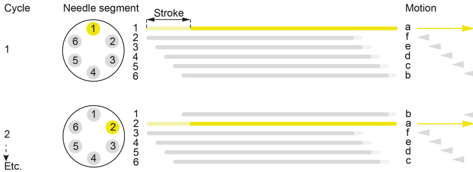
Figure 10.3. Visualization of the motion sequence of the needle segments of the wasp-inspired needle. During the motion, one needle segment (in yellow) moves forward over the stroke distance while the other needle segments (in gray) move slowly backward over one-fifth of the stroke distance in a consecutive manner.
