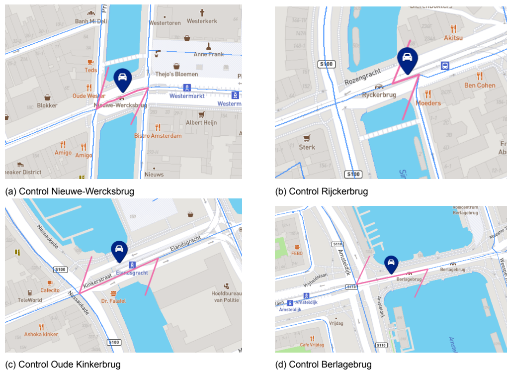
Figure 5.2: Controls and corresponding road links of the 4 selected bridges. In dark blue the activated controls, in pink the selected road links. The half arrow tips on both sides show that the control operates on both directions. In Figure 5.2b and Figure 5.2d it can be seen that the bridge consists of multiple road links. By closing one of the road links, the bridges are still completely closed.
