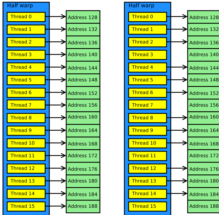
Figure 3.3: Examples of coalesced global memory transactions
