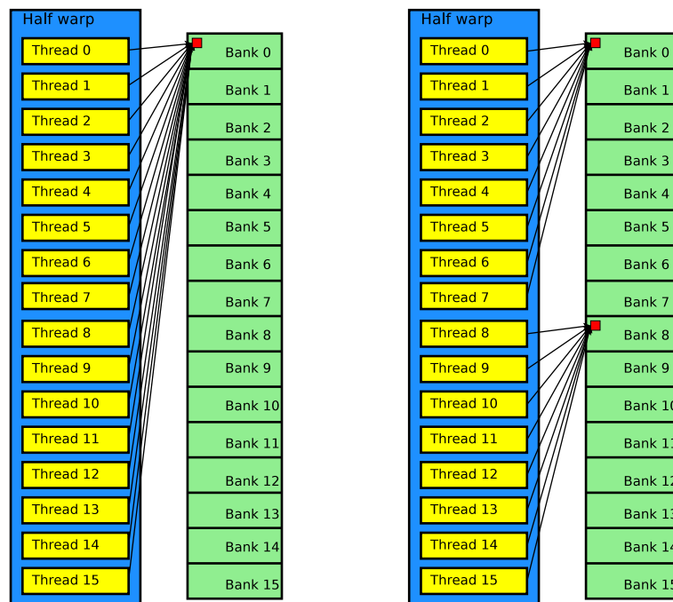
Figure 3.6: An example of how the shared memory broadcast mechanism works: The left access pattern will lead to one single memory transaction, while the right access pattern will lead to two sequential transactions.
