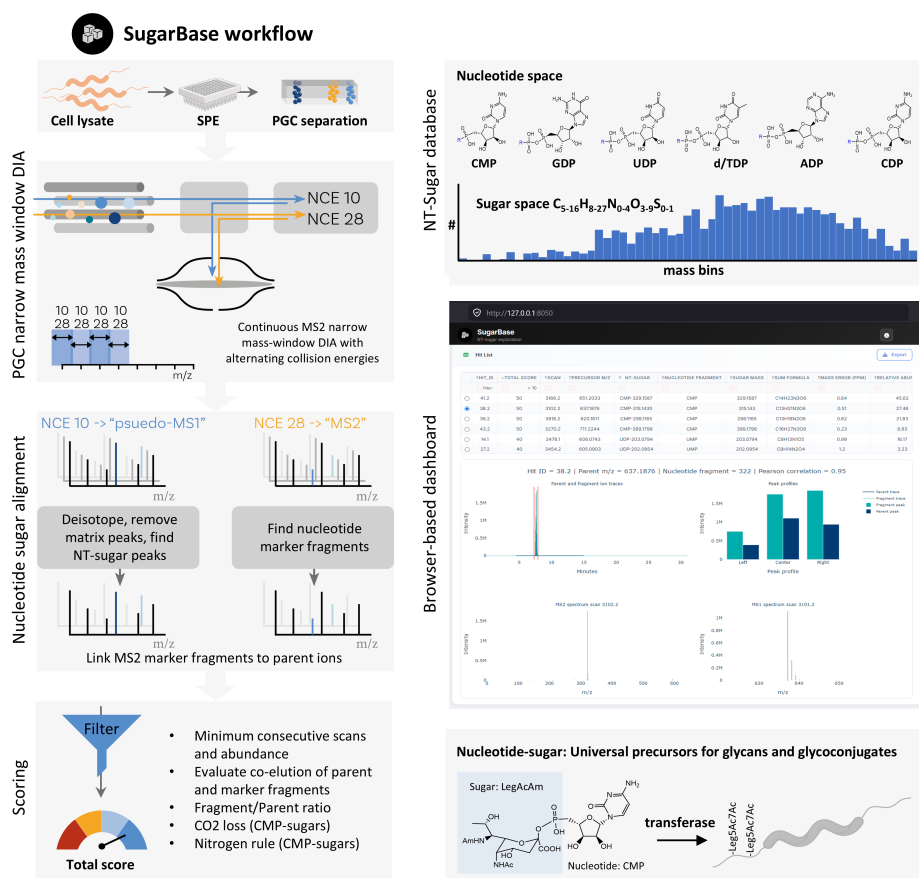
Figure 3.1. SugarBase: mass spectrometry and bioinformatics workflow for untargeted exploration of microbial nucleotide sugar networks. a) Metabolite extracts are analyzed by porous graphitic carbon separation coupled to narrow-window DIA mass spectrometry. Each window is first acquired at low collision energy to record intact precursor ions (pseudo-MS1), followed by higher energy to obtain fragment spectra (MS2). Pseudo-MS1 spectra are deisotoped and filtered, while MS2 spectra are screened for nucleotide marker fragments. Matching scans are linked to identify nucleotide sugars, and precursor ions are assigned using a sugar composition database. Candidates are evaluated based on consecutive detection, co-elution of precursor and marker ions, realistic intensity ratios, and for CMP-linked sugars, CO_2 neutral loss and the nitrogen rule. Identifications can
