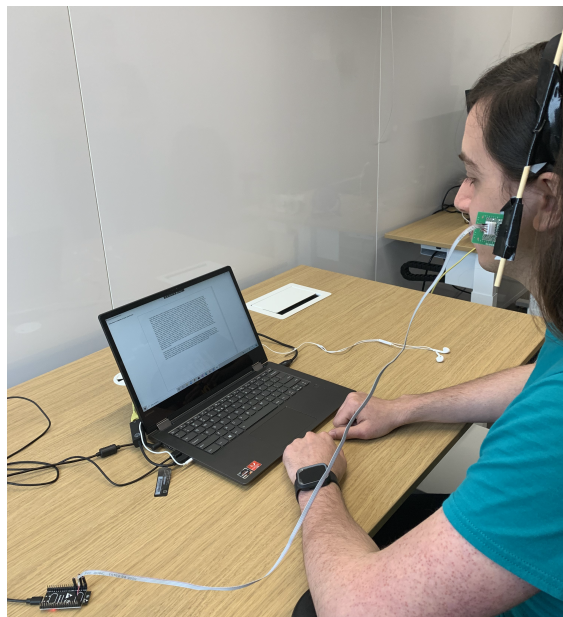
Figure 4. An overview of the experiment setup, with the IR-sensor shown on the participants head. Screenshots of the experimentation text-reader software can be found in Appendix G. Note: this is not the room the experiment took place in.
