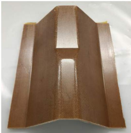
(a) Formed shape before post-consolidation process
