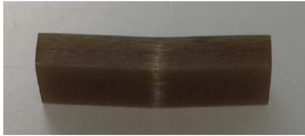
Figure 5.2: Longitudinal tensile failure in SBS test specimen
