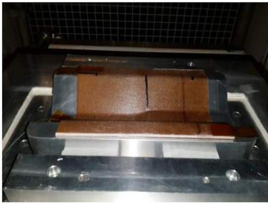
(a) Formed shape fixed on the metal mould
