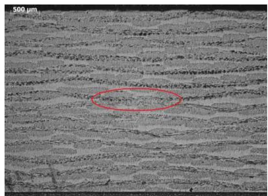
(b) Cross section of co-consolidated laminate in run n°6 (2)
