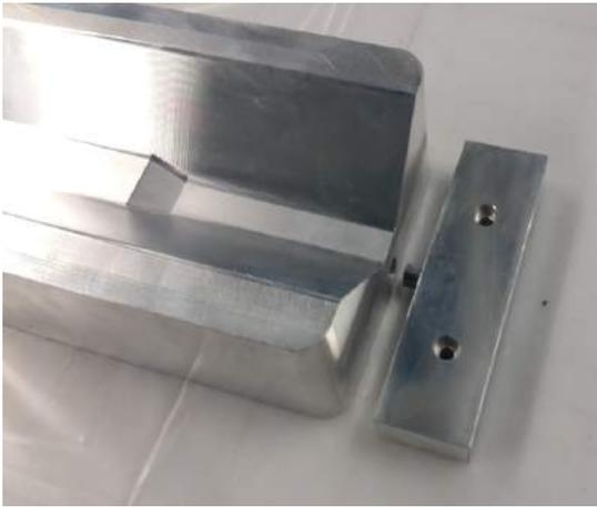
Figure 3.12: Constraining block preventing metal mould from being released from mounting plate
