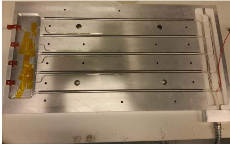
Figure 3.17: Heating plate with five heating elements
