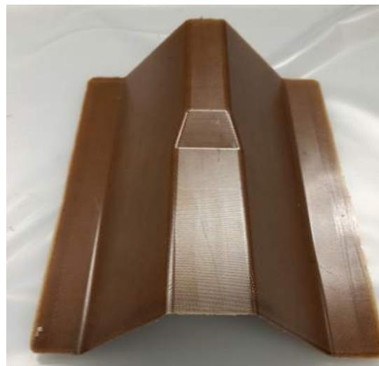
(b) Formed shape after post-consolidation process
