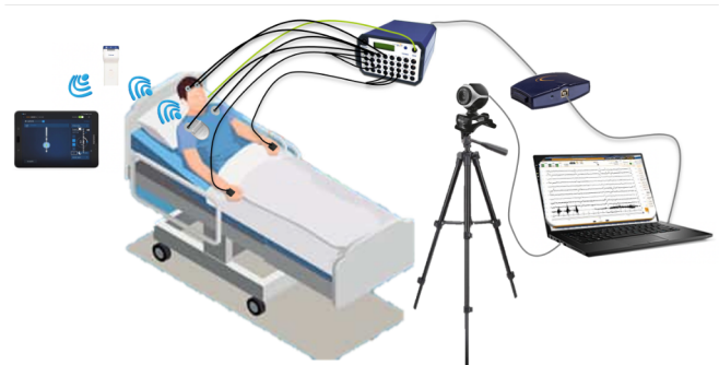
Fig. 1: Schematic overview of the experimental setup. On the left the wireless communication via a relay device between the implanted Percept and the tablet programmer. On the right the external data running through the TMSi amplifier to the laptop. A webcam videotaped the recording.
