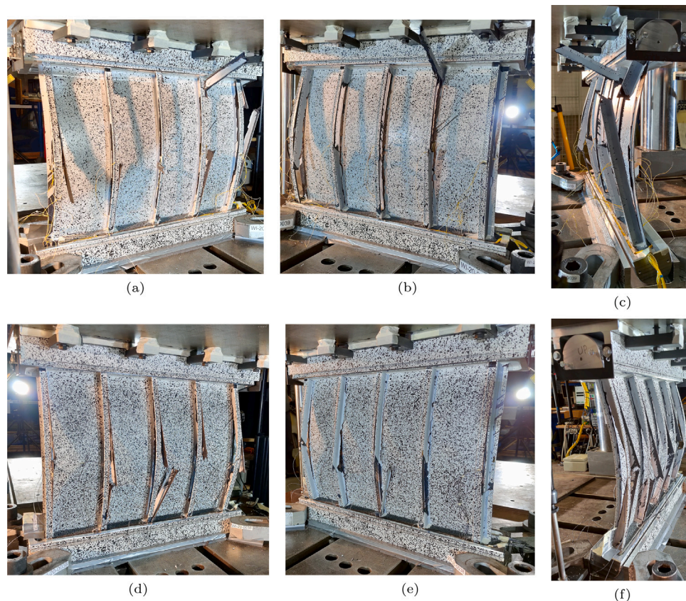
Fig. 15. Post-failure photos: (a) panel 1 left-view; (b) panel 1 right-view; (c) panel 1 side-view; (d) panel 2 left-view; (e) panel 2 right-view; (f) panel 2 side-view.
