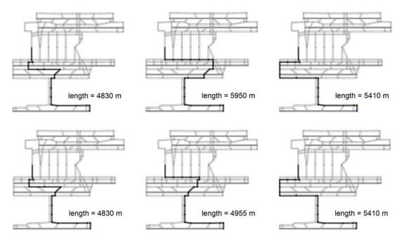
Figure 5. Alternative routes from last exit runway 08 to Gates T for branch and bound algorithm (top) and Dykstra based algorithm (bottom) for the basic Atlanta model
