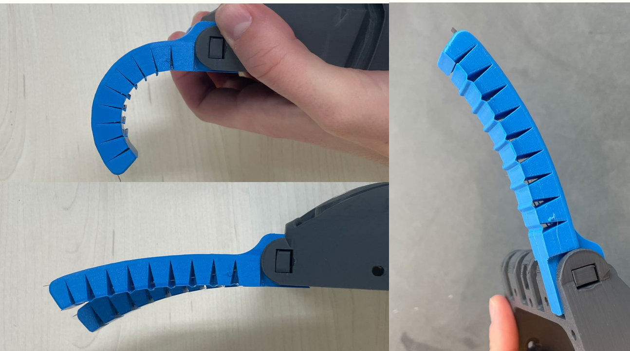
Figure 61: Comparison fingers with and without bottom layer
