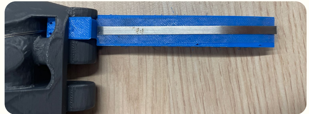
Figure 50: Added spring steel on top of the finger part
