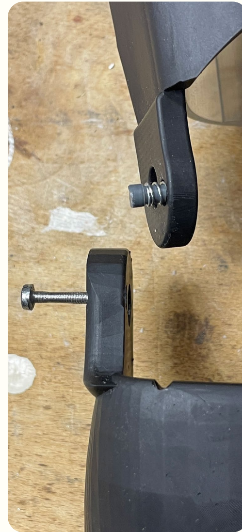
Figure 96: hand and wrist component with integrated clamping system
