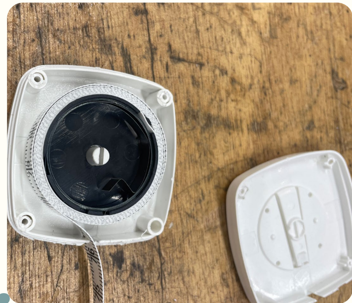
Figure 14: Tape measure mechanism
