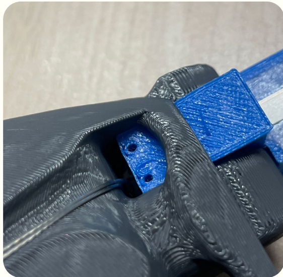
Figure 49: wire blocked due to the angle
