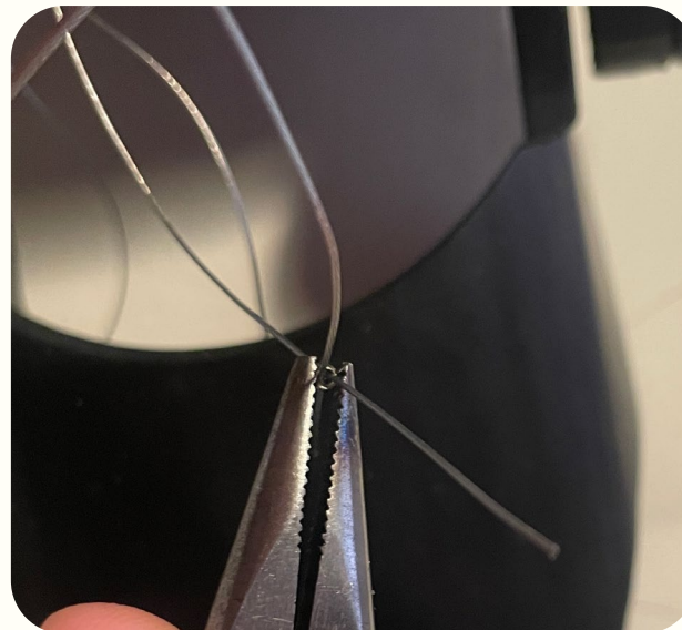
Figure 106: Crimp bead attaching two wires
