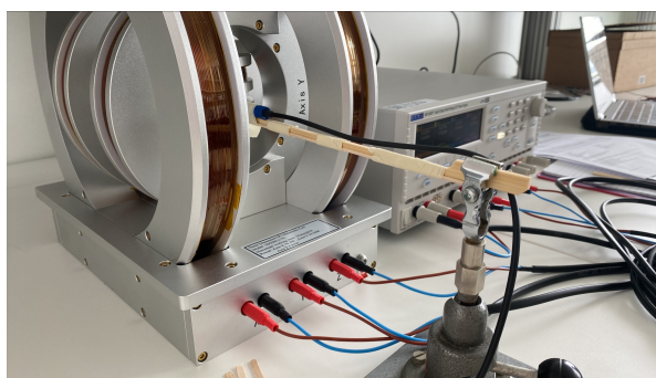
Figure 3.2: Setup of the Gauss meter probe in the 3D Helmholtz coil
