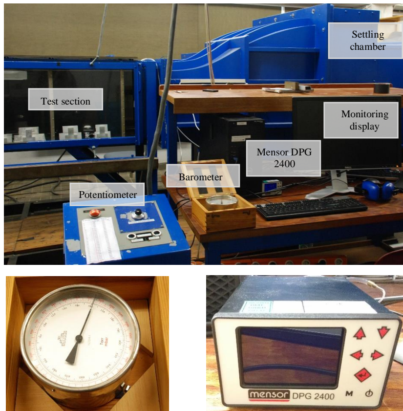
Figure 3.2. M-tunnel various parts, sensors and freestream velocity control and display (top). Details of analog barometer to measure static ambient pressure (bottom left) and the Mensor DPG 2400 digital pressure gauge to measure freestream dynamic pressure (bottom right)
