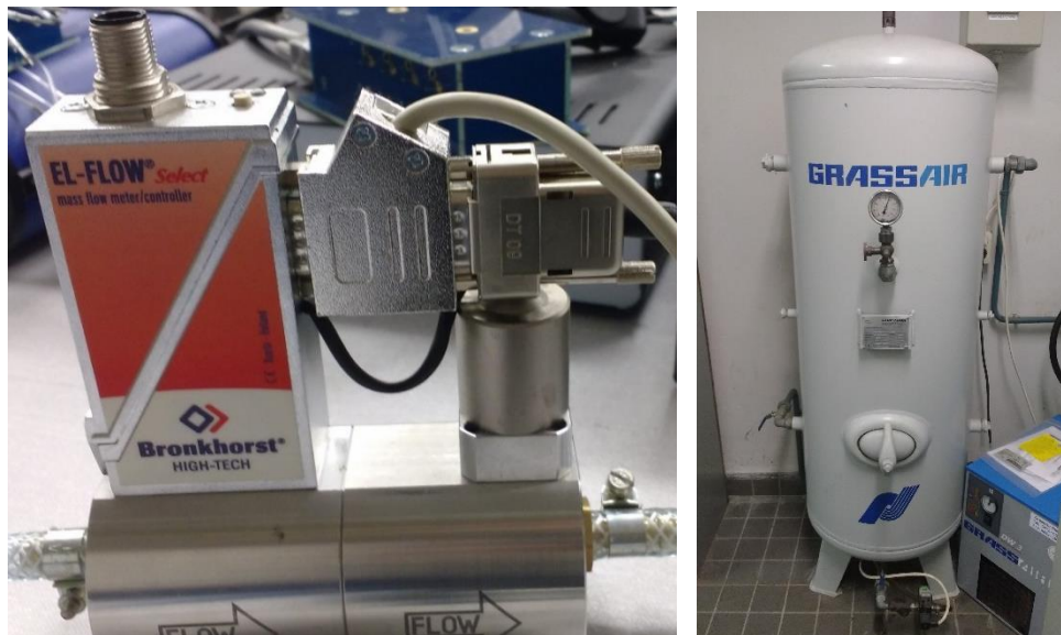
Figure 3.4. Bronkhorst F-202-AV used in the experiments (left). It is calibrated for air and limited to a maximum volumetric flow rate \dot{m} = 260 \text{ l/min} . Grassair compressor that provides the air supply at a pressure P \sim 10 \text{ bar} (right).
