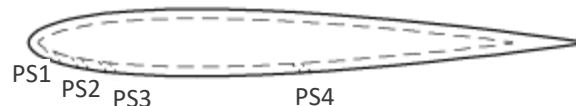
Figure 3.5. Sketch of the model adapted from (Lanzillotta, et al., 2017). PS1 refers to the cooling holes row in the pressure side located at a 5% of chord length distance from airfoil's leading edge; PS2 at 10%, PS3 at 15% and PS4 at 50%.
