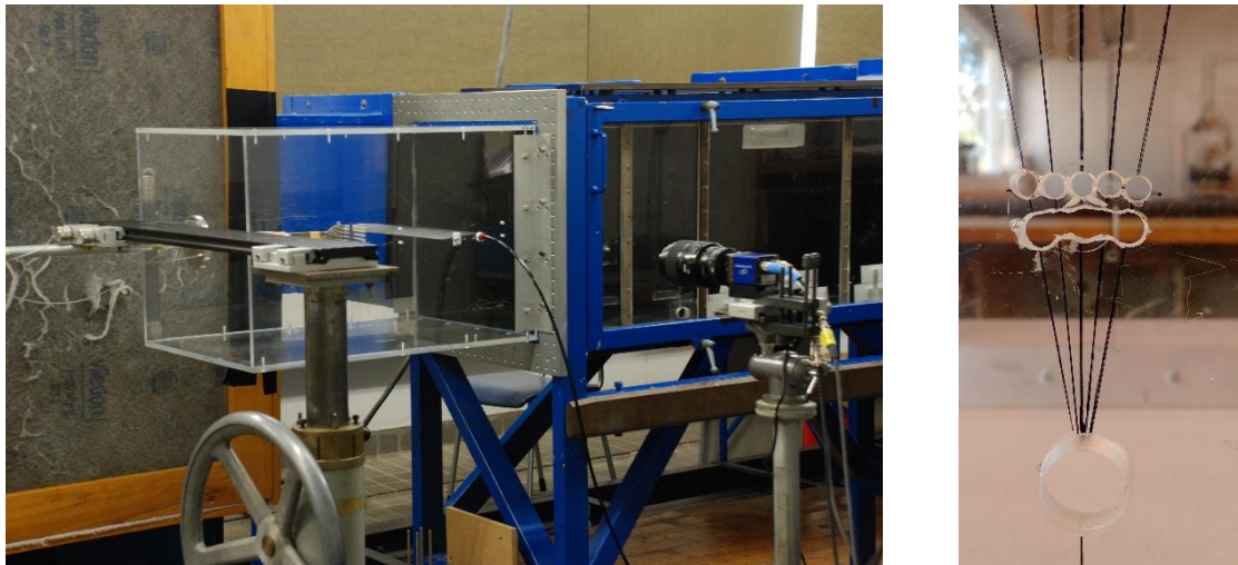
Figure 3.1 M-tunnel test section with the plexiglass test section attached to it and the airfoil model inside (left). Detail of the holes in the plexiglass test section to fix the airfoil at five different angles of attack (right)
