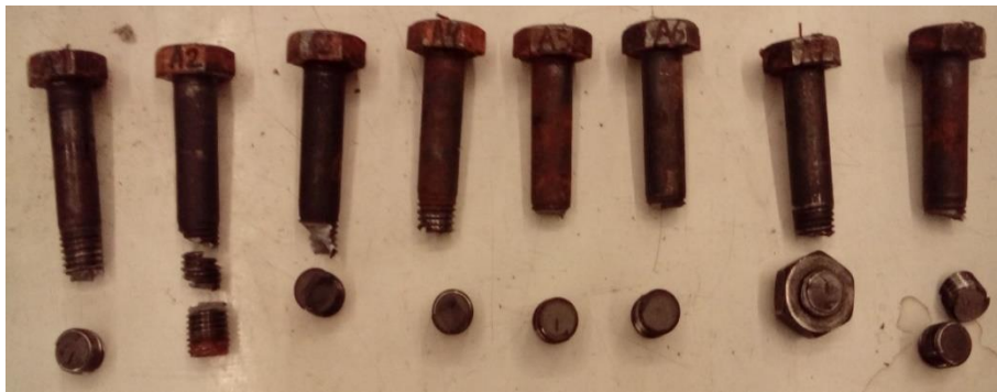
Figure 5.26: Broken bolts (B series)
