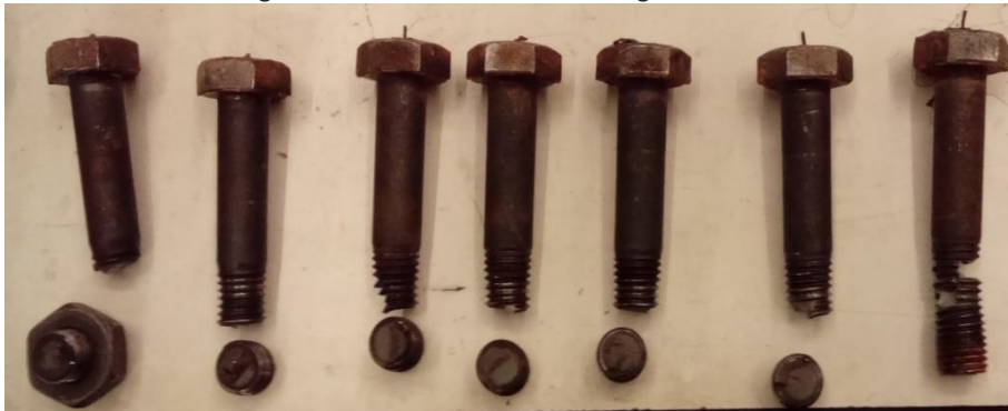
Figure 5.25: Broken bolts (A series)
