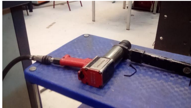
Figure 4.16: Pneumatic tightening device
