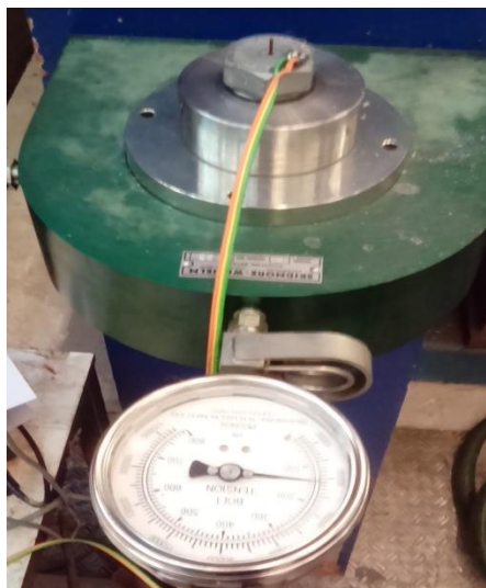
Figure 4.20: M24 bolt (B2) in tensile force instrument
