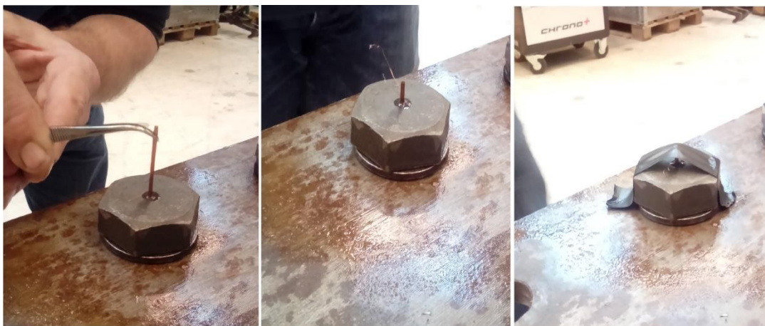
Figure 4.13: Installation of the strain gauge
