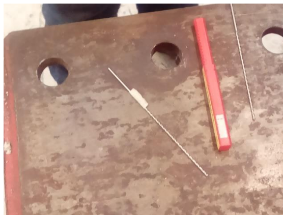
Figure 4.6: Drilling bit with a tape at the length of 40 mm
