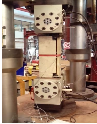
Figure 5.24: UTM for material testing of the bolts
