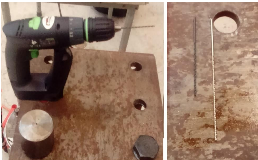
Figure 4.5: Drill and drilling bits used in drilling process
