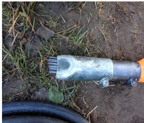
Figure 5.6: Paint removal tool
