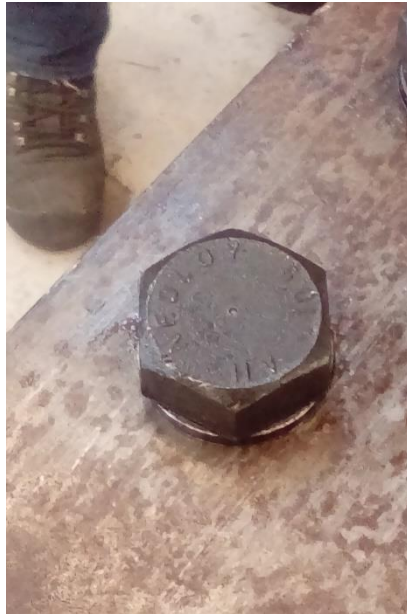
Figure 4.9: Hole on the head of the bolt
