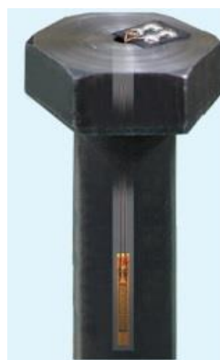
Figure 3.11: Strain gauge embedded [37]
