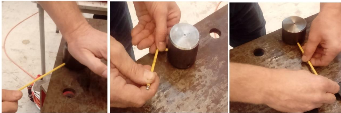
Figure 4.4: Clamping of the hexagonal die on the head of the bolt
