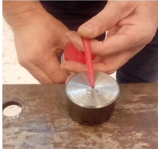
Figure 4.22: Injection of drilling oil
