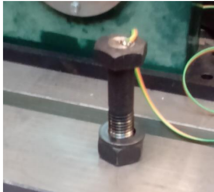
Figure 4.19: M24 bolt (B1) with implanted strain gauge
