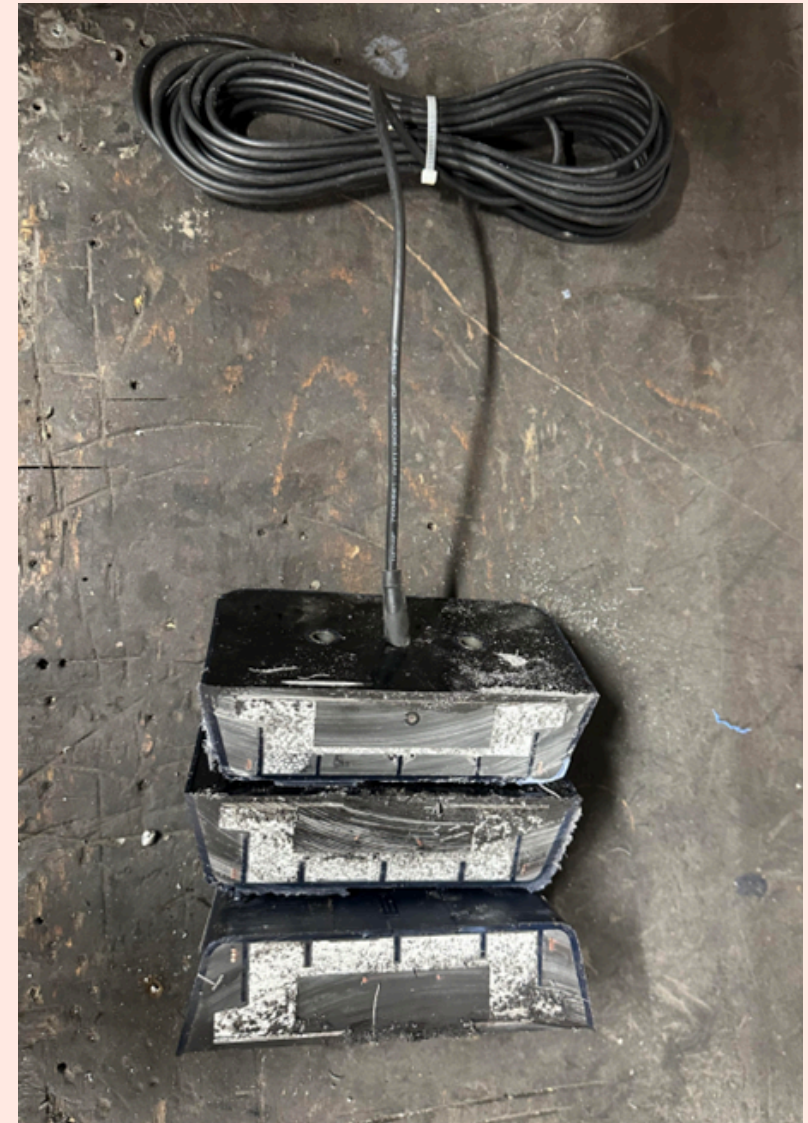
Figure 21: One antenna of three after MiterSaw preparation for shredding
