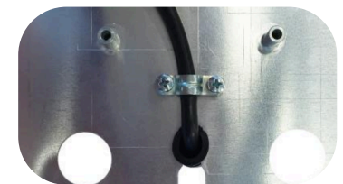
Figure 5: Strain relief holding the cable down
