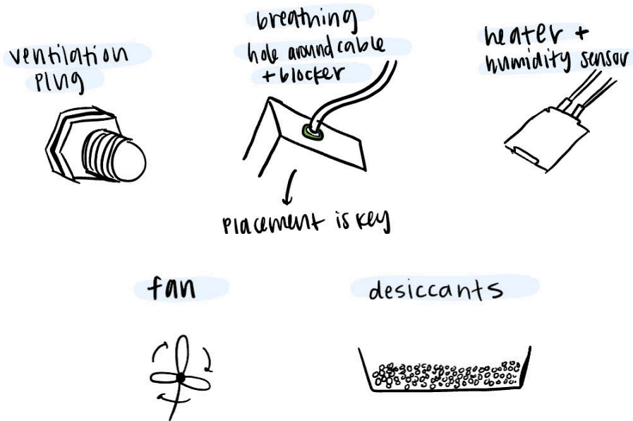
Figure 47: Brainstorm drawings of temperature stabilization concepts
