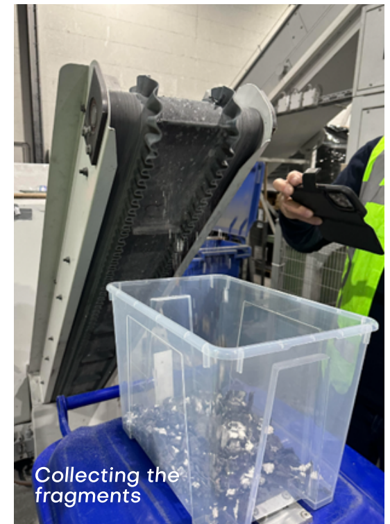
Figure 22: The shredding process of the antennas going through the fine shredder
