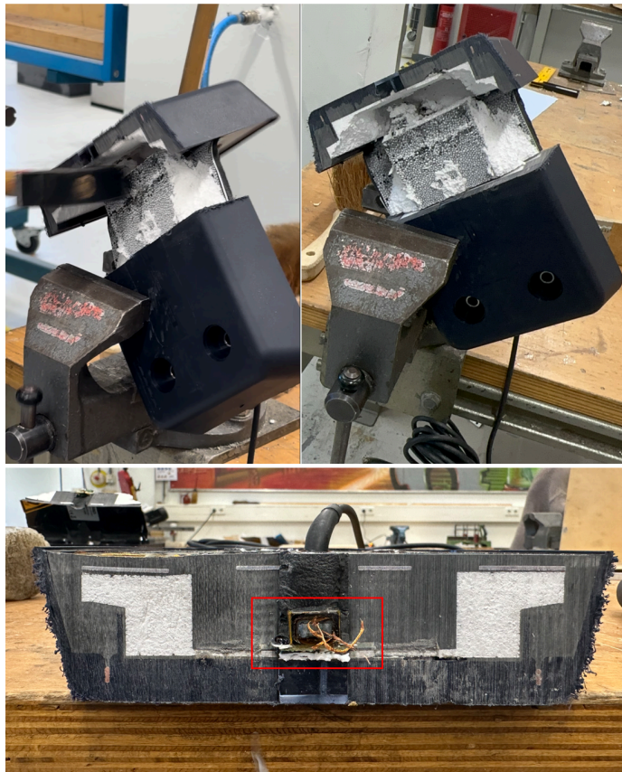
Figure 18: Dismantling of the antenna through bandsaw and hammer
