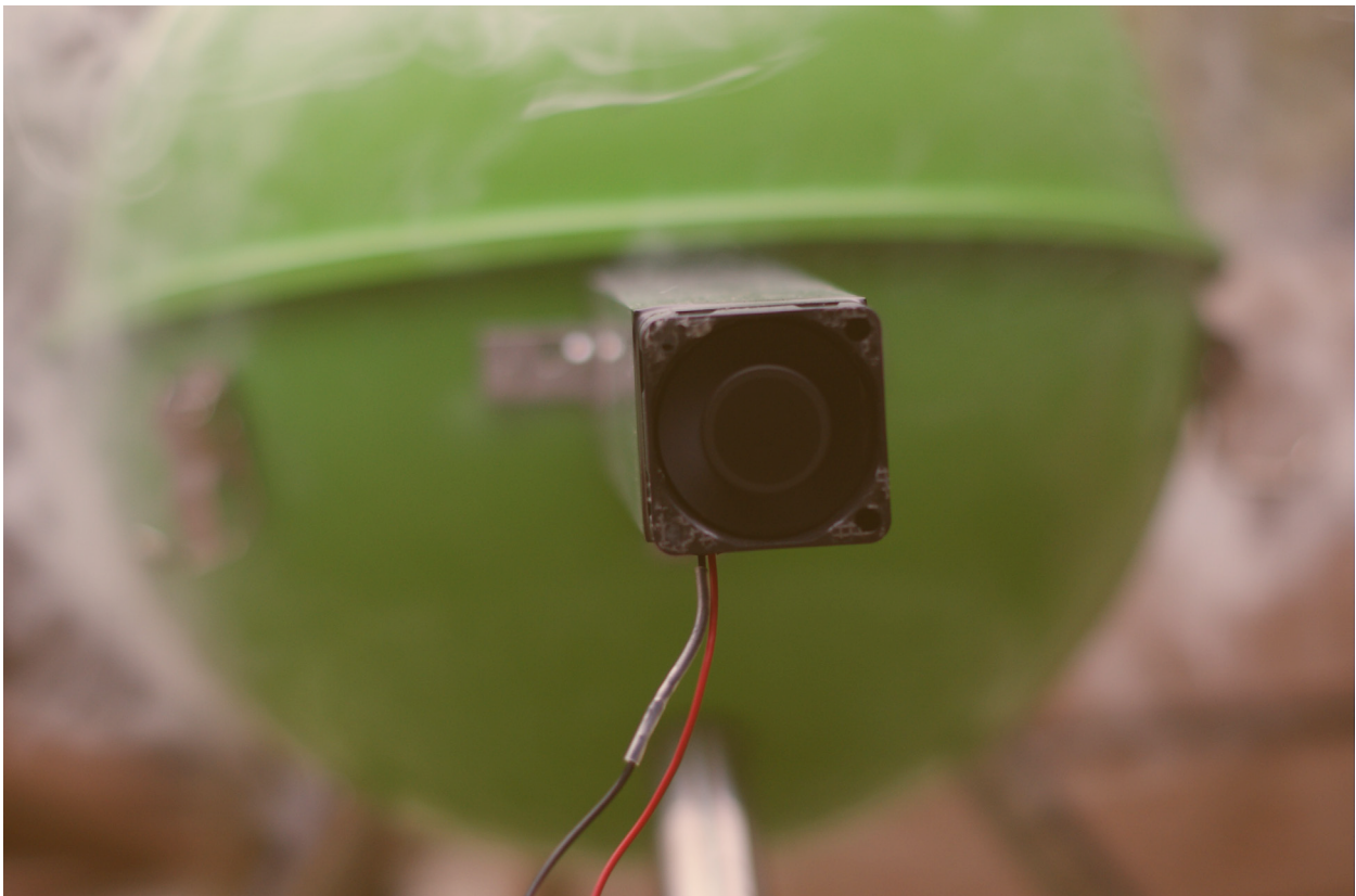
Figure 23. Arduino powered fan that adds more oxygen to the barbecue but also cools it down
