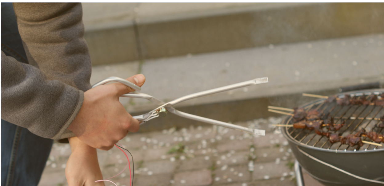
Figure 28. Barbecue tongs prototype that can measure thickness of food
