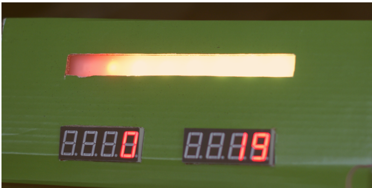
Figure 31. LED prototype that resembles the barbecue flow and associated temperatures
