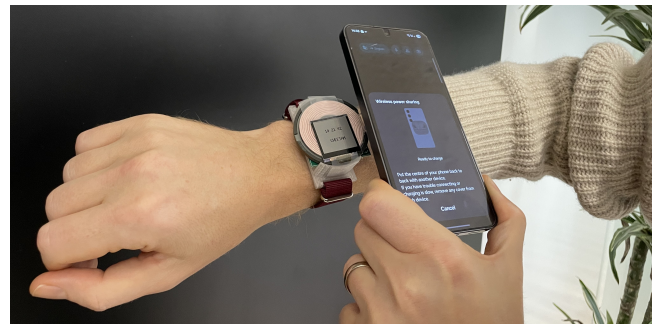
Figure 1: Demonstration of a user charging a Cheetah-enabled battery-free smartwatch within seconds via a smartphone using Qi wireless power transfer system.
