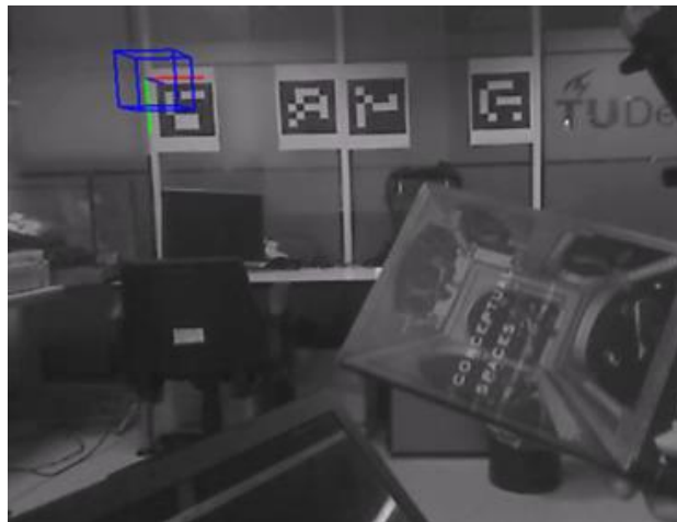
Figure 5.1 Multiple markers are used to avoid Aruco becoming 'lost' as much as possible. It is important that their relative distance, corresponding to a file read by Aruco holding these distances, is accurate enough for good camera pose estimation.
