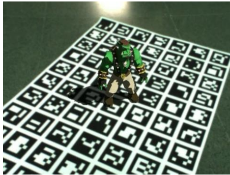
Figure 7.2 A marker that is generated by Aruco. It uses printable boards with multiple markers to increase accuracy and make it more robust against occlusions.
