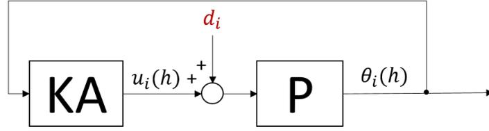
**Figure 2-8:** Kuramoto model with matched input disturbance
