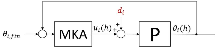
**Figure 3-9:** Error feedback system with the predicted final orientations as reference
