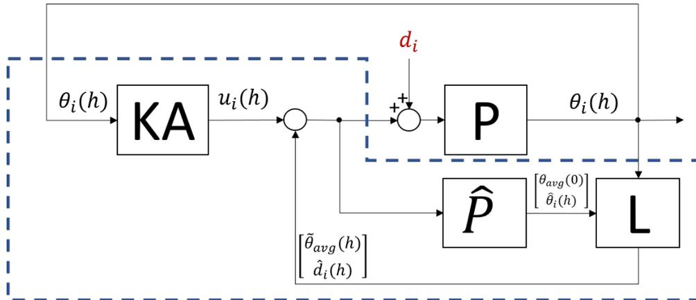
**Figure 4-5:** One step ahead predictor and deadbeat control with average state reference
