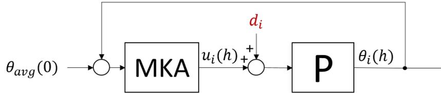
**Figure 3-1:** Error feedback system with the initial average orientation as reference
