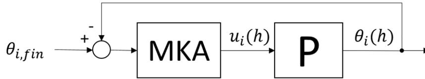
**Figure 3-5:** Error feedback system with the predicted final orientations as reference
