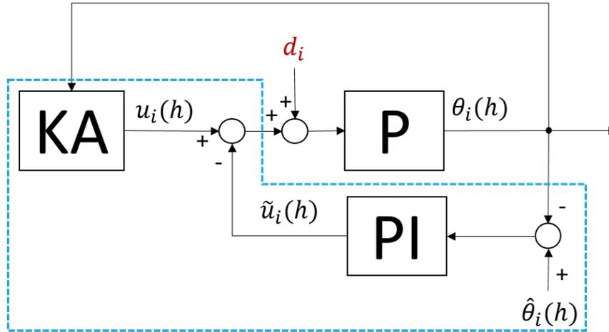
**Figure 5-2:** The system with autonomous reference trajectories and PI-control. The controller is indicated by the dashed blue line
