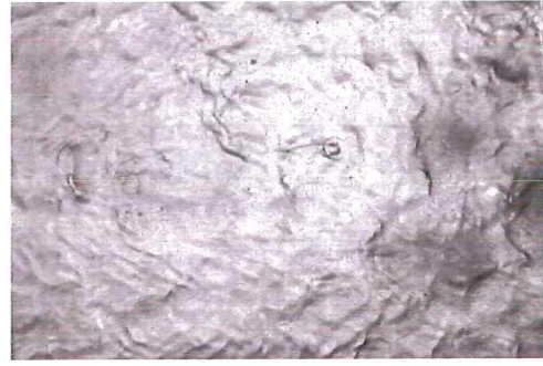
Figure 6.2: Rippled surface for flow in a horizontal pipe, at a superficial liquid velocity of 1.2 cm/s and a superficial gas velocity of 28 m/s. The width of the picture is 2.4 cm and the height is 1.6 cm. The flow is from right to left.
