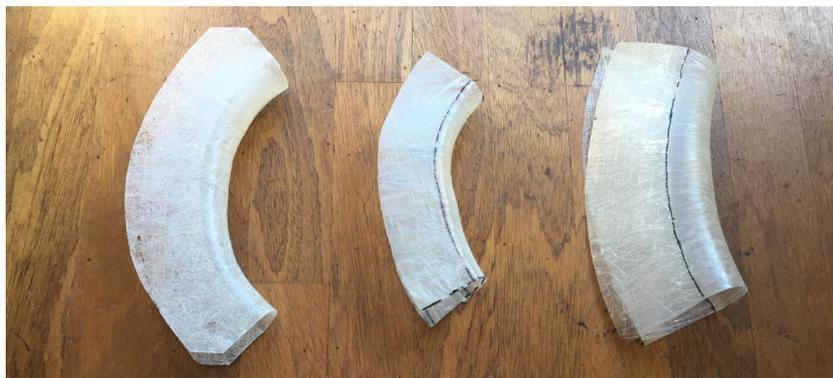
Figure B.8: Three prototypes that resulted from the lamination process: (from left to right) CSM with small transverse and longitudinal radius and wide flanges, cross-ply directional fiber mat with small transverse and longitudinal radius but limited flange width, cross-ply directional fiber mat with two large radii and wide flanges.
