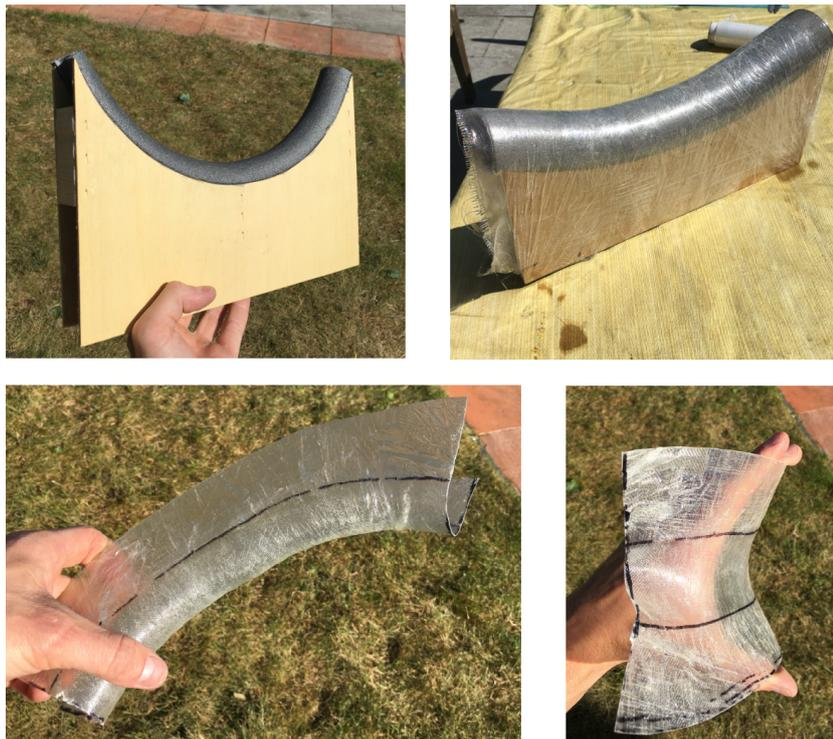
Figure B.7: The manufacturing process for creating the first bi-stable shell prototypes required a mould (top left) and a fiberglass lamination process (top right). The undeformed and inverted state are depicted in the bottom left and bottom right pictures respectively.
