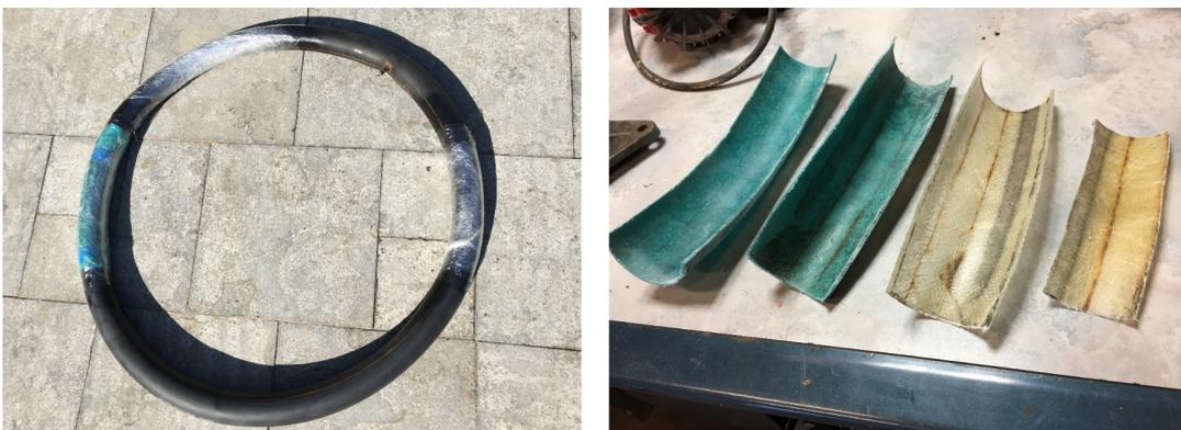
Figure B.6: An attempt to fabricate double curved shell sections, representing the crease sections of the shell. On their own, no stable inverted state was noticed.
