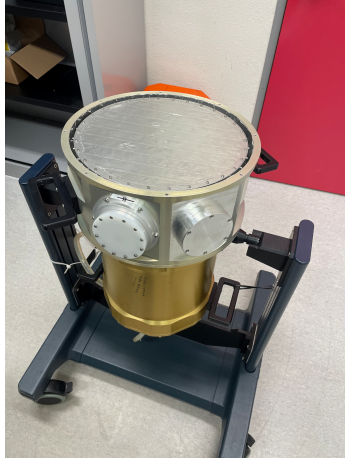
(d) A picture of the cryostat at SRON. When in use the cryostat would be flipped around as to have the gold colored cryogen reservoir assembly on top of the silver colored working area assembly.
