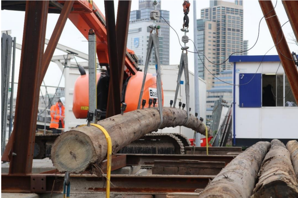
Figure 2.11, Four-point bending experiment on timber quay wall foundation pile.
