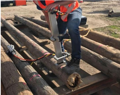
Figure 3.10, IML micro drilling performed on all piles after the bending experiment was executed.
