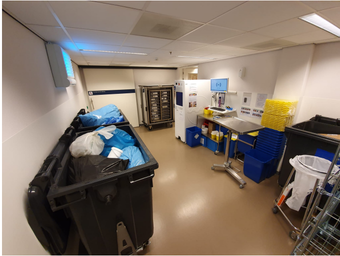
Figure 4.9: This is the 'dirty' /waste room. On the left hand side you see the big black containers in which the garbage bags with disposable material is thrown. The instrument nets are placed in the metal cart in the back of the picture. On the right hand side you see the Pharmfilter TONTO and the blue needle box container.
