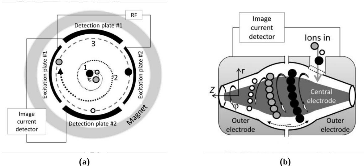
**Figure 2-4:** Two types of mass analyzer incorporating an FTICR technique: **(a)** A standard setup using ion cyclotron resonance (ICR), and **(b)** the more compact version applying ICR Orbitrap [35].
