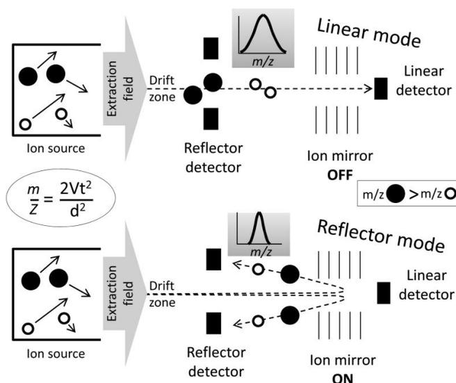
**Figure 2-3:** Two modes of the Time-of-Flight (TOF) mass analyzer: linear and reflector mode [35].
