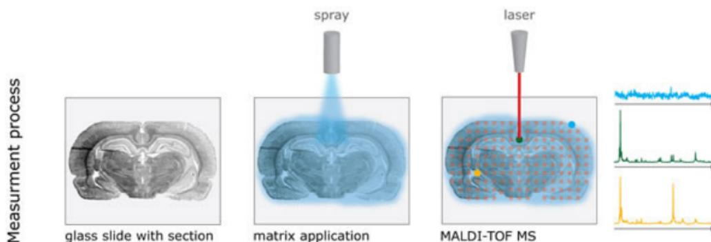
**Figure 2-2:** Visualisation of a typical MALDI-MS process. The application of the chemical matrix can be seen together with the placement of the discrete spatial points determining the pixels of the IMS image. Each pixels contains its own mass spectrum [28].
