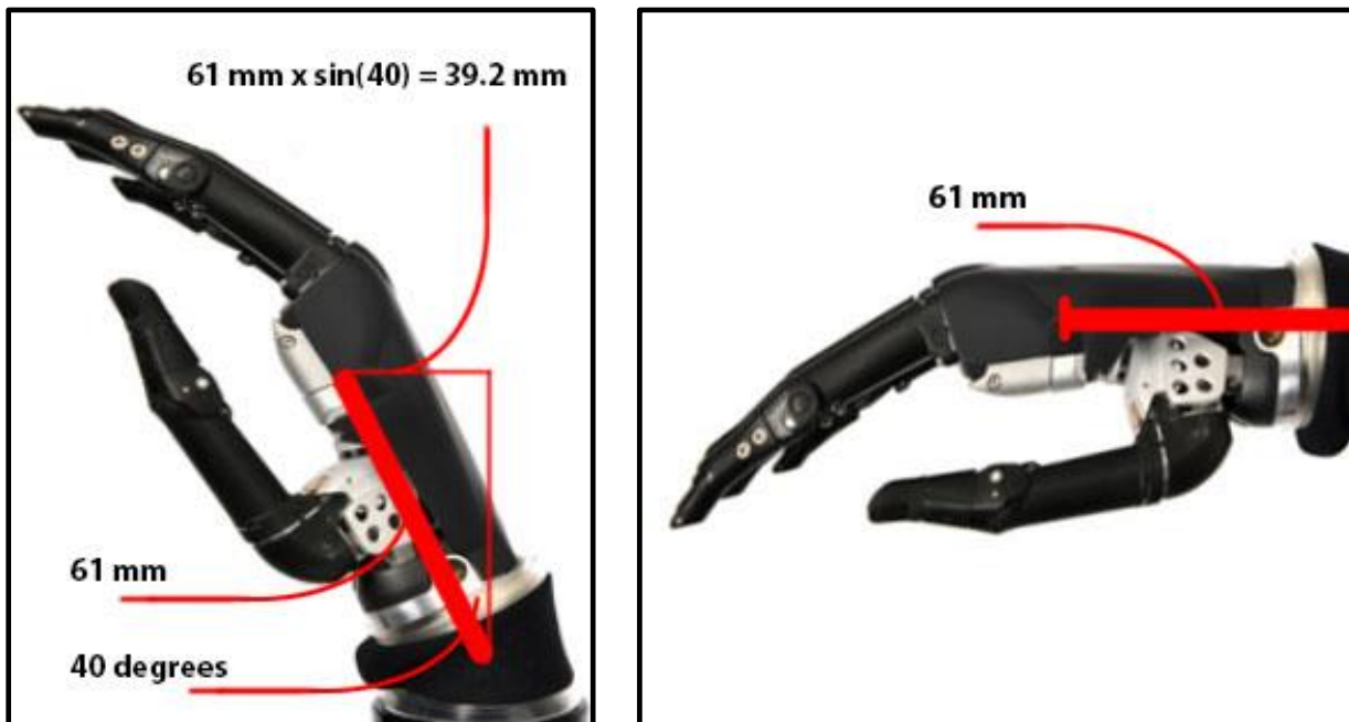
FIGURE 2. REPRESENTATION OF THE MOMENT ARMS CONCERNING THE ESTIMATION OF THE MAXIMUM REQUIRED TORQUE. ON THE LEFT; THE LARGEST POSSIBLE MOMENT ARM FOR ROTATION IS SHOWN USING THE CENTER OF MASS OF A HEALTHY HUMAN HAND [43] AND THE MAXIMUM NEEDED AMOUNT OF FLEXION FOR ACTIVITIES OF DAILY LIVING [40]. ON THE RIGHT; THE LARGEST POSSIBLE MOMENT ARM FOR FLEXION/EXTENSION. THIS RESULTS IN A REQUIRED MAXIMUM TORQUE OF APPROXIMATELY 200 N·MM FOR ROTATION AND 300 N·MM FOR FLEXION/EXTENSION.
