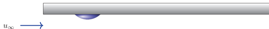
Figure 6.3: Basic setup of a single droplet attached to a flat surface, blown by an imposed free-stream airflow u_\infty .
