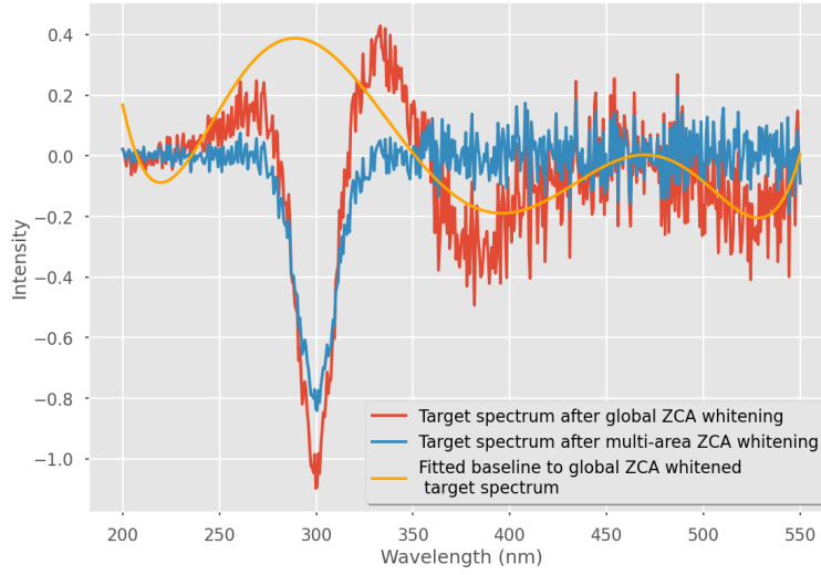
Figure 3.11: Spectra of the target pixel after using global ZCA whitening and multi-area ZCA whitening, and the baseline that is fitted to the target spectrum after global ZCA whitening, pixels used as observations.
