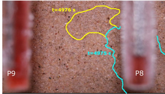
Figure 3.6: Zone around pipe tip in test B25_245 s just before ( t=4975 s) and during ( t=4976 s) second group detachment.
