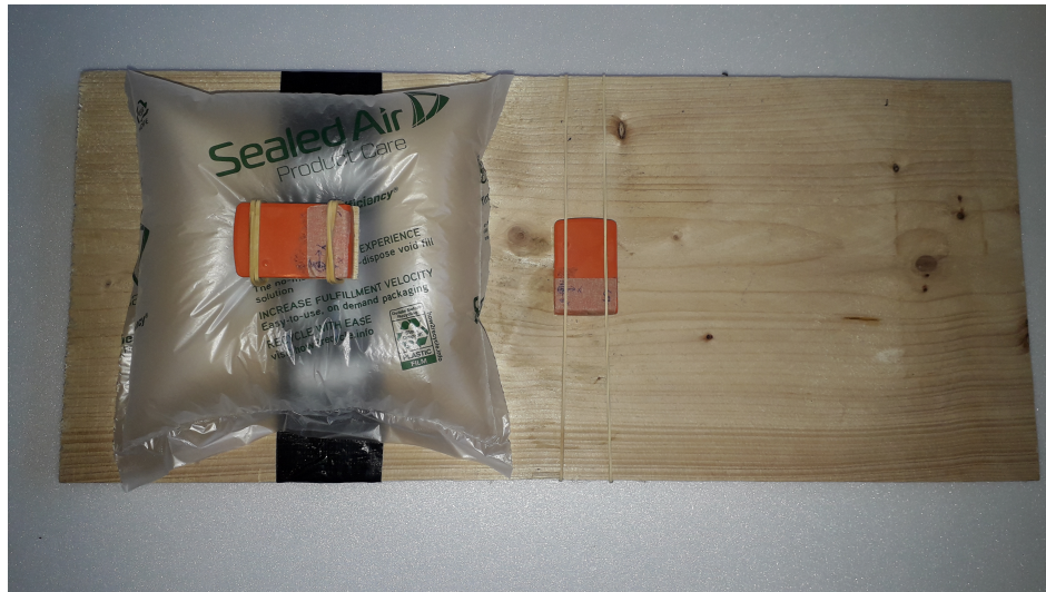
Figure 5-4: The setup of experiment 3 allows mutual movement between the sensors.
