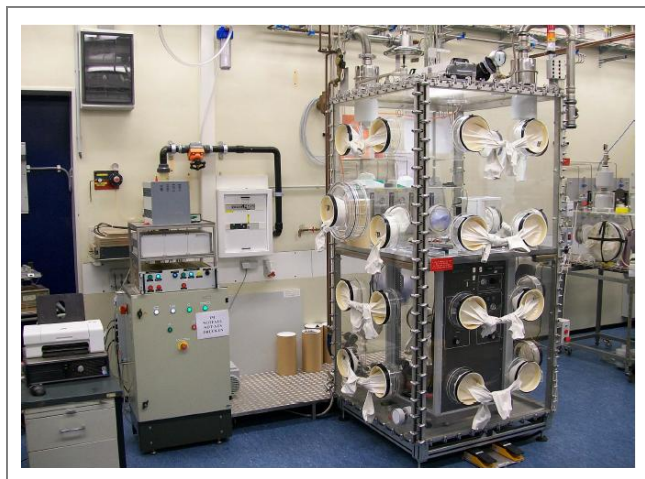
Figure 1. A drop calorimeter installed in an alpha-tight glove box in ITU. The labelled box on the left contains electronic parts of the calorimeter that were excluded from the glove box.
