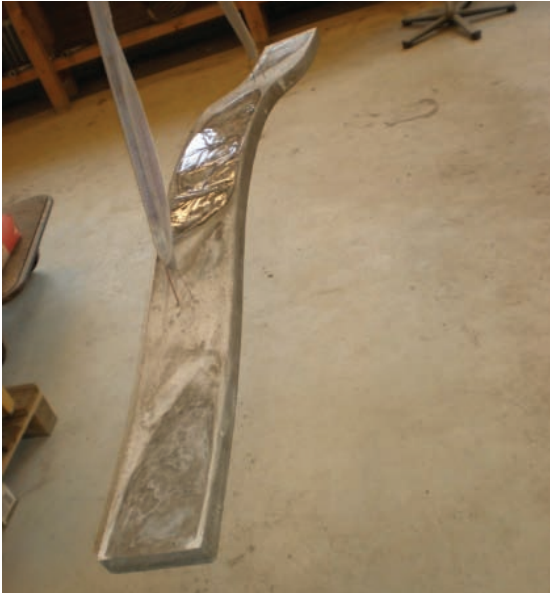
Figure 8: Single-curved Element 5 after demoulding
