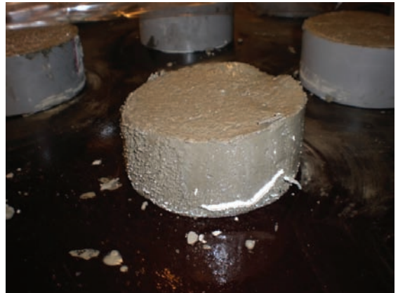
Figure 6: Consistency testing 45 minutes after casting (Mixture M2)
