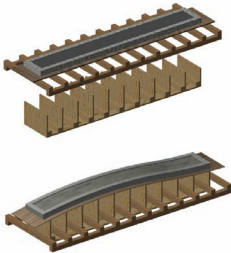
Figure 4: Two production steps for single-curved test specimens: a) casting in horizontal position, b) mould after deforming
