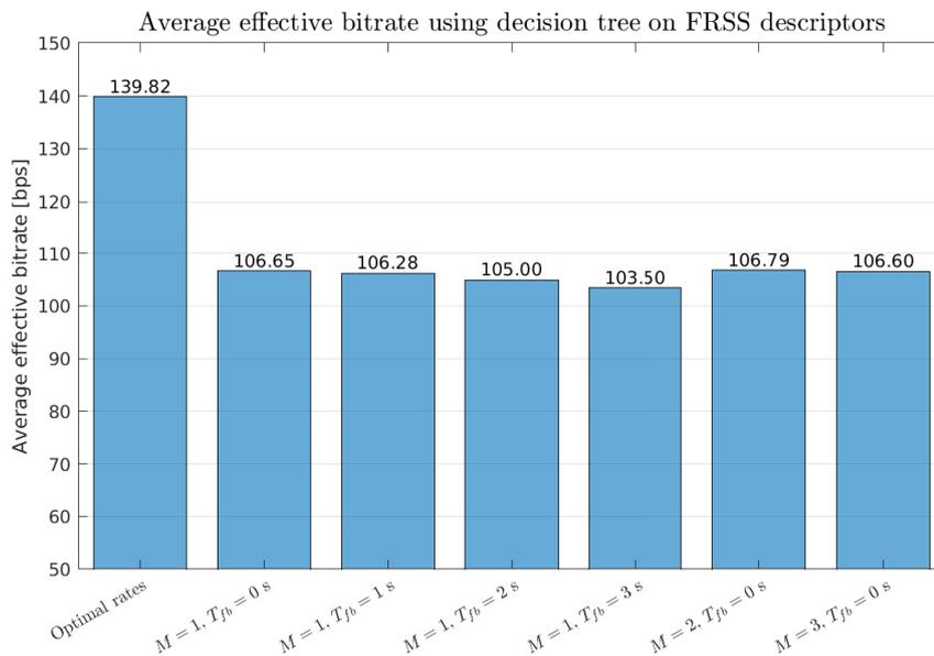
Figure 4.10: Average effective bitrate using decision tree classifier on FRSS descriptor values for various feedback delays and lookbacks.
