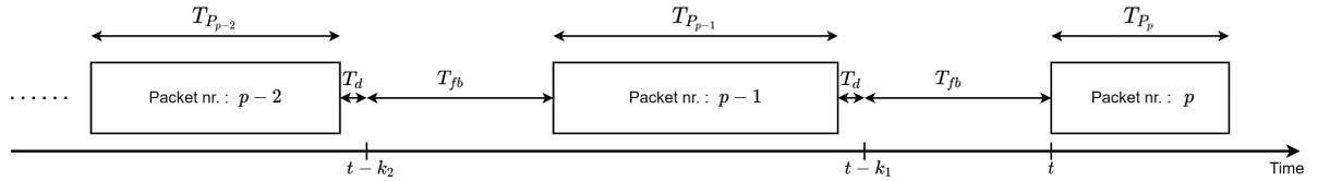
Figure 4.3: Schematic overview of link adaptation structure in time, seen from the transmitter side.
