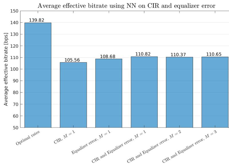
Figure 4.11: Average effective bitrate using neural network classifier on CIR and equalizer error.
