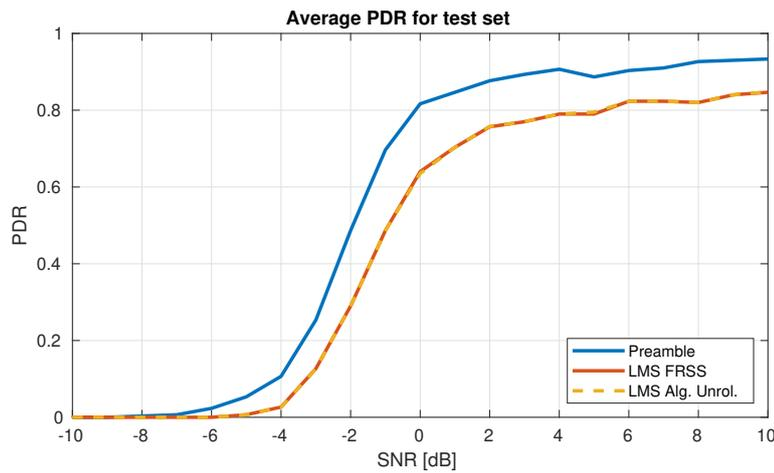
Figure 5.2: Average PDR of detection preamble, LMS filter with FRSS step size parameter and LMS filter with  $\mu = 0.0033$  found using algorithm unrolling.
