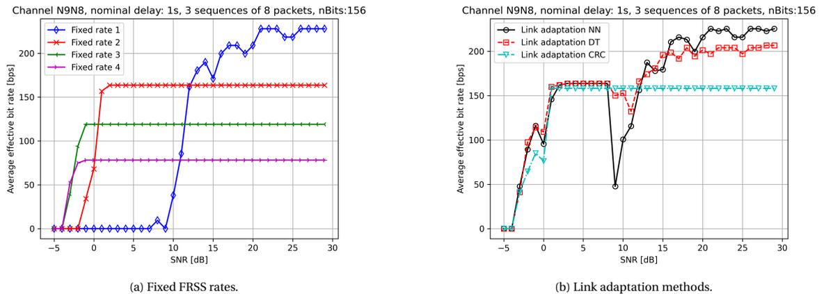
Figure 4.15: Performance of ML link adaptation techniques compared to fixed FRSS rates in channel N9N8.
