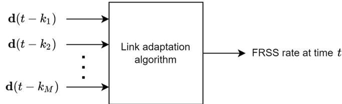
Figure 4.4: Schematic overview of link adaptation algorithm inputs and output.
