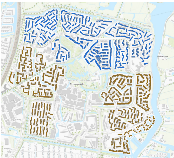
Figure 8: technology coverage for this scenario; low temperature heating networks are blue while the high temperature networks are brown.
