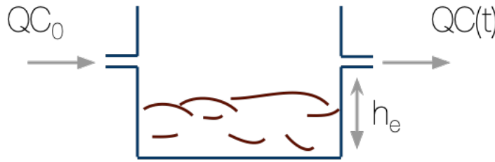
Figure D.1: Mass balance of solids in the septic tank
