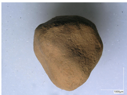
(a) FeOx coated sand grain
