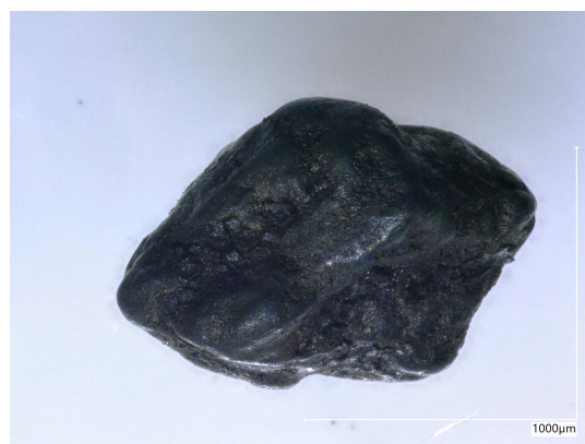
(b) MnOx coated sand grain
