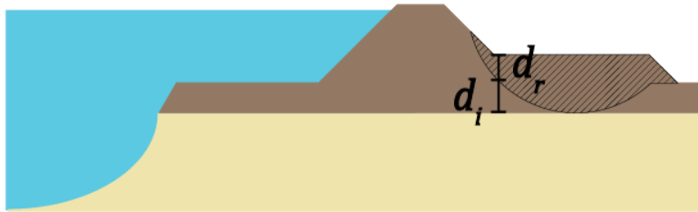
Figure 4.14: Intact and remoulded blanket layer thickness
