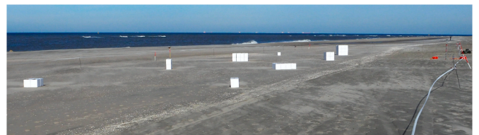
Fig. 3. The set-up at one of the days (12-10-2018), testing the effect of building width and height. Note: scale model configuration, orientation and location changed between all experiments.
