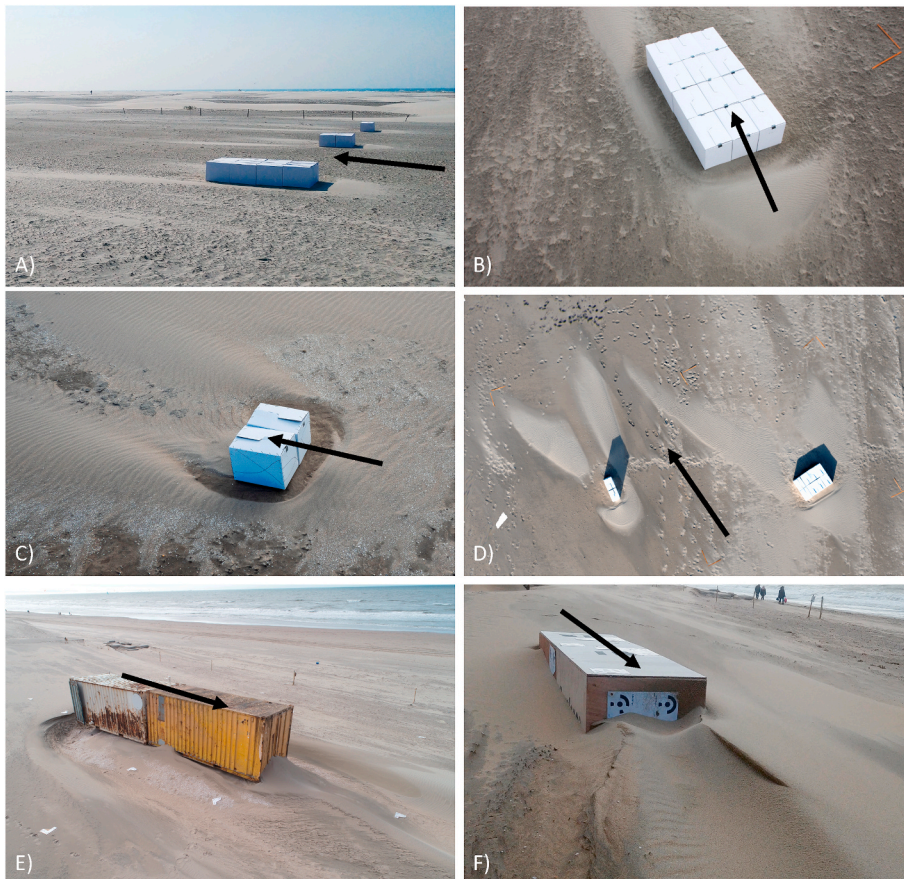
Fig. 12. Examples of deposition around scale models, with arrows indicating the (dominant) wind direction. A) Small scale models of different length, with upwind deposition and deposition tails visible as lighter areas (29-05-2018). B) The nearest small scale model of photo A from another angle. C) Deposition with a considerable elevation difference (23-10-2018). D) An orthophoto of deposition (12-10-2018). E) The full-scale model of the 5-week experiment, showing deposition, erosion and undercutting under the upwind side of the container (11-03-2020). F) The small scale model of the 5-week experiment, half-buried and with a deposition tail downwind of the model (11-02-2020).
