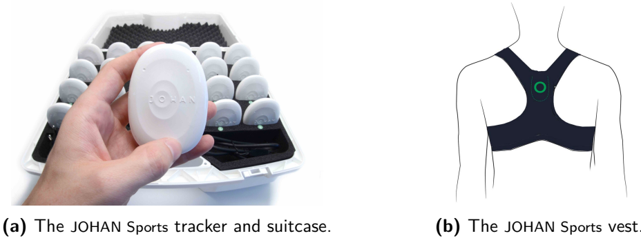
Figure 1-1: The JOHAN Sports tracking device comes in a suitcase that serves as a charging station. It is worn in a vest on players' upper back, causing the least discomfort while playing. Figures by courtesy of JOHAN Sports.
