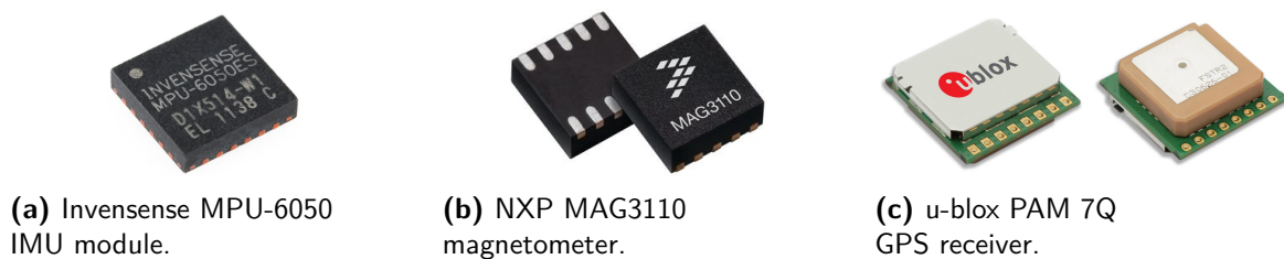
Figure 2-5: The sensors that are contained in the JOHAN Sports tracking device.
