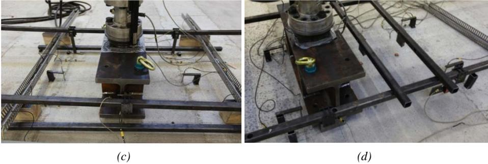
Fig. 4.3 Instrumentation of the top side of the deck slab: a) BB15 (P1M); b) BB10 (P1J); c) BB16 (P2M); d) BB6 (P2J).
