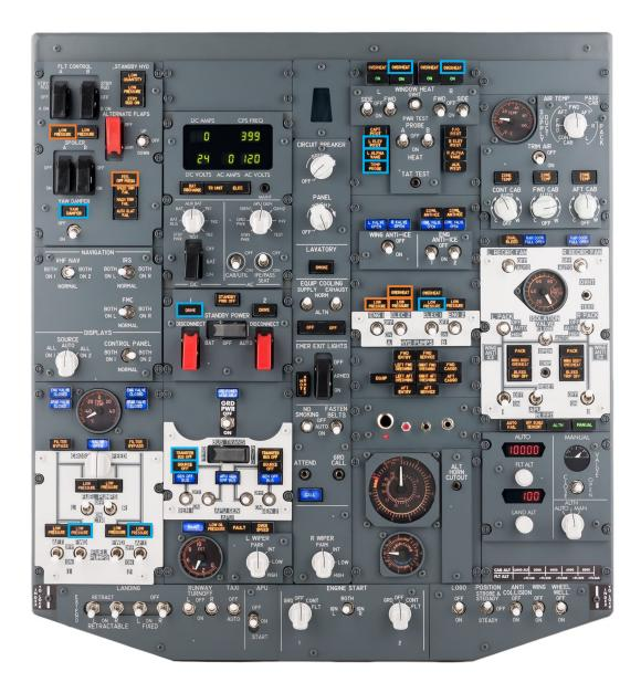
Figure B.6: The overhead panel for the Boeing 737-8. Indicated in blue are the lights illuminated during the drive shaft failure, whereas the indications are in orange for the hydraulic leak failure
