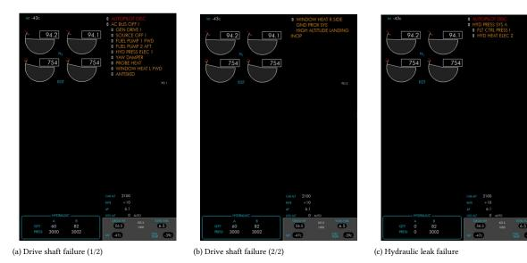
Figure B.7: Overview of EICAS messages presented to the participant for the drive shaft failure in (a) (messages page 1) and (b) (messages page 2) and the hydraulic leak failure in (c)
