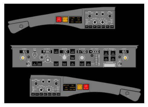
Figure B.1: The master caution system is located on both sides of glareshield panel. As a reference, the glareshield panel location within the flight deck can be seen in Figure B.4 [35]
