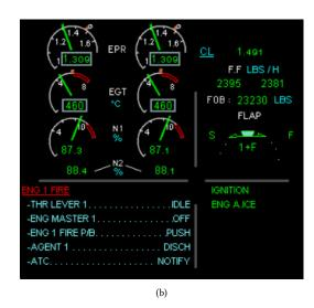
Figure 2.1: The NNC representation as on the Boeing 787 ECL [8] in (a), and as part of ECAM in (b)
