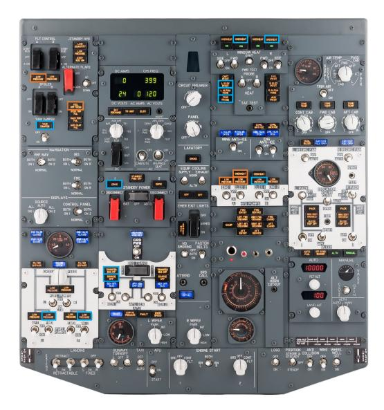
Fig. 9: The overhead panel of the Boeing 737-8. Indicated in blue are the lights illuminated during the drive shaft failure, whereas indications in orange represent the illuminations experienced during the hydraulic leak failure
