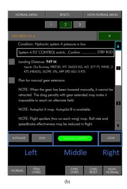
Figure 7.4: The three zones of the automation and checklist handling bar. Zone left handles automation, zone middle allows the pilot to supervise automation (a) and checklist progress (b), and zone right is responsible for removing checklists from the non-normal menu once completed
