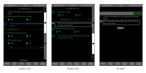
Figure 7.2: The Source Off NNC displayed on the ECL is shown in (a) and (b) for page 1 and page 2, respectively. The non-relevant overridden steps are in blue and make the display relatively cluttered when compared against the AECL in (c)
