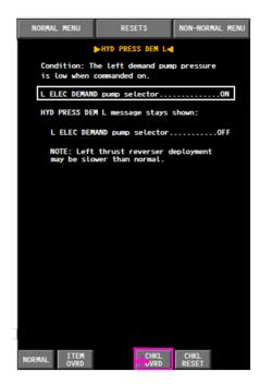
Figure 2.6: Example of a checklist presented on the Boeing 787 ECL [8]. The HYD PRESS DEM L checklist was opened from the non-normal menu displayed in Figure 2.5 [8]
