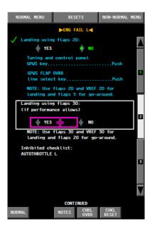
Figure 2.23: Example of a completed and an uncompleted conditional line item in the ENG FAIL L checklist. The completed closed loop conditional line item shows how now no longer relevant steps are overridden, whereas the uncompleted open loop conditional line item provides an example of how the pilot is required to select 'YES' or 'NO' in order to continue [8]
