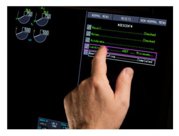
Figure 2.32: Manipulation of an ECL with the integrated touchscreen technology on the Boeing 777X
