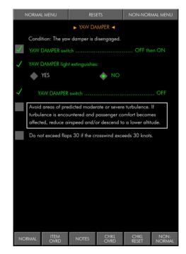
Figure 7.5: The step-by-step process as on the Boeing 787 ECL. Note that the first three steps would have been automatically complete items are presented to the pilot, a reduction of 60% with automation
