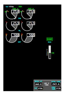
Figure 2.2: A schematic organisational overview of the EICAS display and its indications on the Boeing 787 [8]
