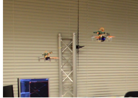
Fig. 1: Two pocket-drones (40 g each) flying autonomously in a real-world indoor environment using only on-board sensing and processing.
