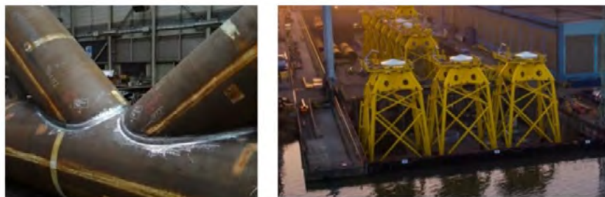
Figure 1. Traditional Welded joints used in multi-membered jacket offshore wind turbine support structures
