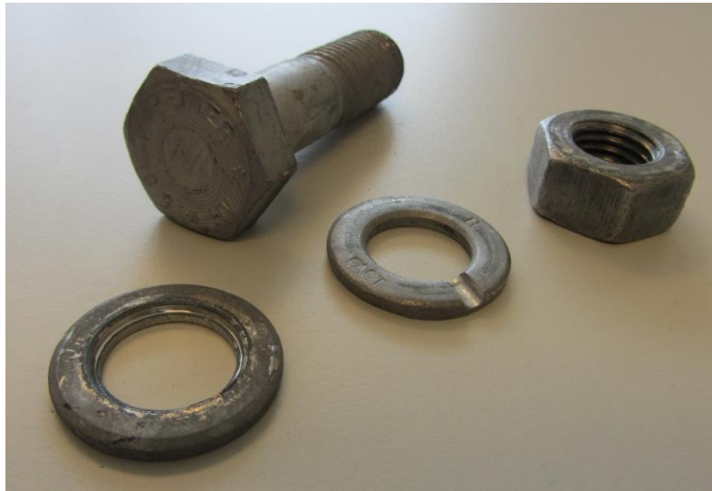
Figure 43 Fastener assembly of injection bolt with bolt, washers and nut
