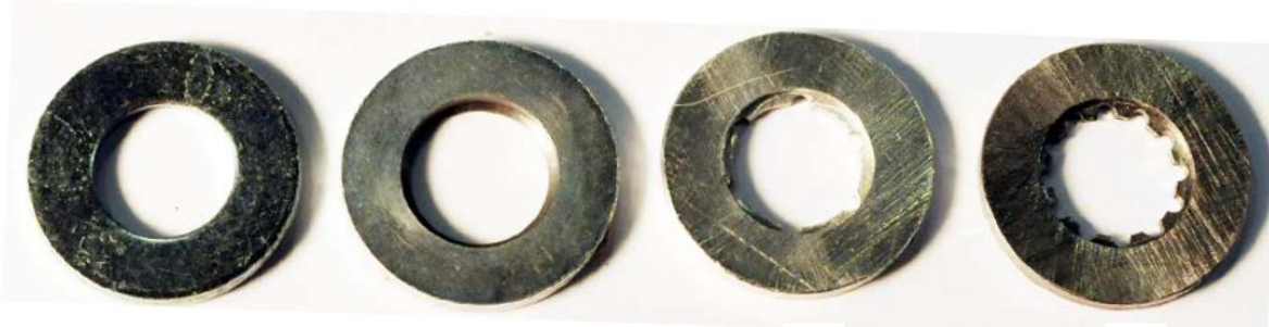
Figure 14 Bolt head washer designs investigated in research on Sikadur 30 and RenGel resin IBC in FRP structures [28]
