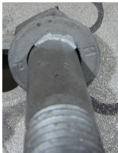
Figure 70 Sikadur-30 failed injection at bolt head washer interface
