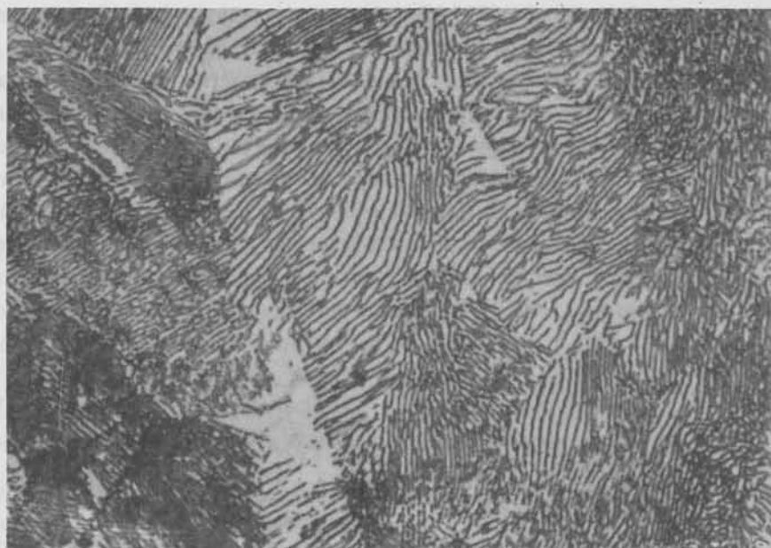
Figuur 3.5. Lamellaire perliet; etsing \text{HNO}_3 in alcohol (1600 \times ).
