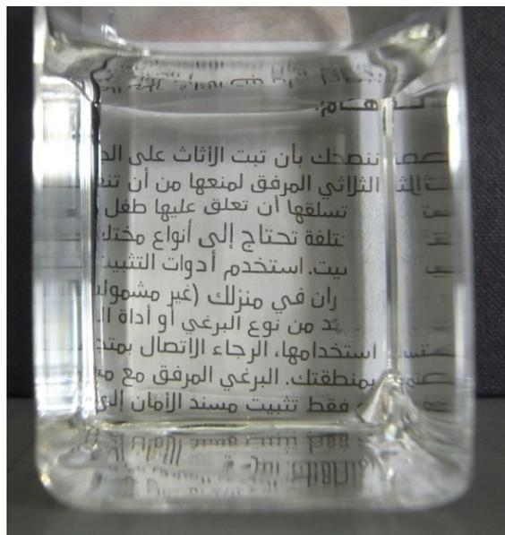
Figure 7.1. A photograph in daylight of a 40x40 mm<sup>2</sup> square cell containing an RFG gel which had been irradiated with two, 10 mm diameter crossed X-ray beams each with an average dose of ~20 Gy. For a fluorescent image of the same gel see figure 7.8.
