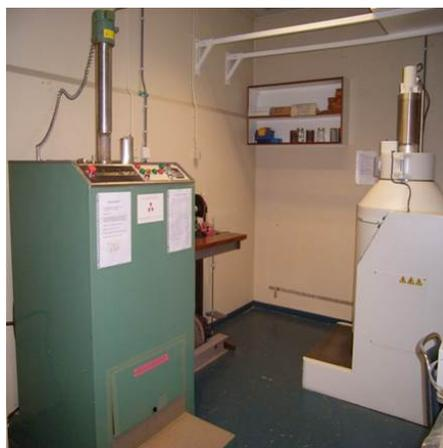
Figure 2.4. Cobalt-60 irradiators gammacell 200 from Atomic Energy of Canada (left) and 220 from Nordion (right).
