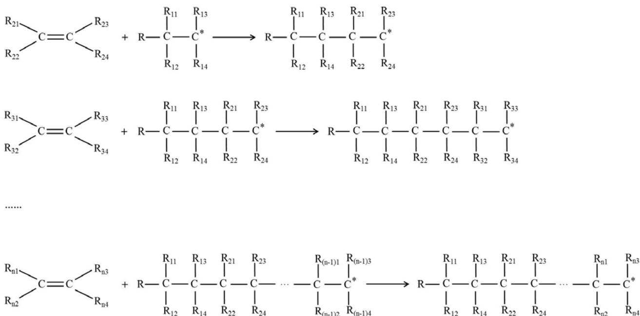
Fig. 2. Schematic presentation of chain growth.
