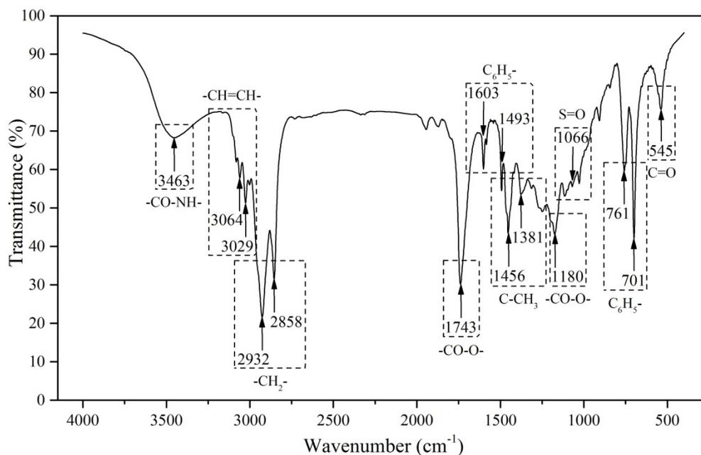
Fig. 8. Functional groups of typical bio-bitumen product.
