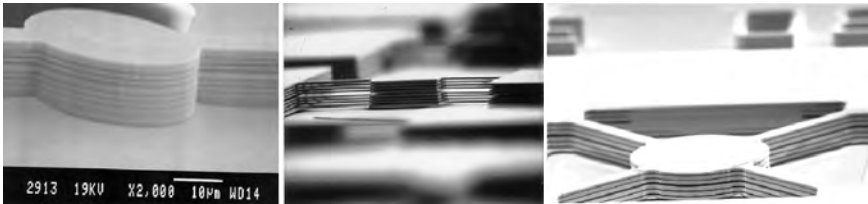
Figure 1.6: SEM views of monolithic tunable Fabry-Perot filters based on InP/air-gap layers. (image reprinted from [12])
