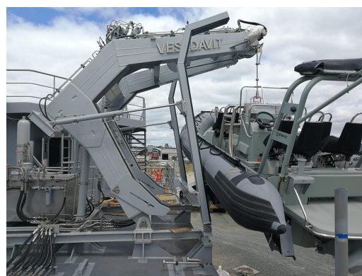
Figure 2.1: Vestdavit davit system and rescue craft
