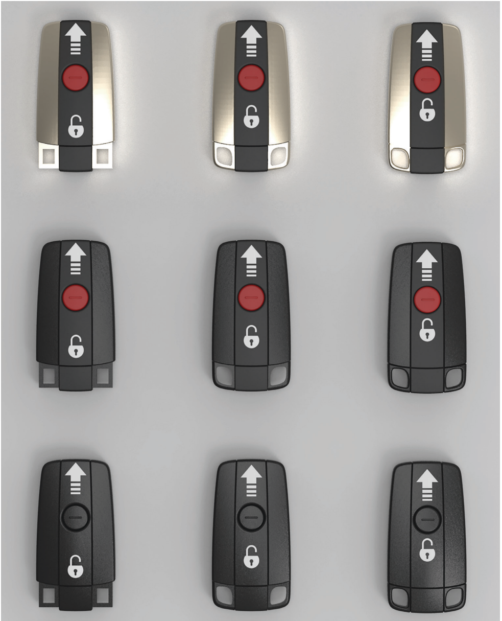
FIGURE 31. REMOTES SYSTEMATICALLY MANIPULATED IN VISUAL UNITY THROUGH PROXIMITY (X-AXIS) AND VARIETY THROUGH COLOURFULNESS (Y-AXIS). DECREASING THE DISTANCE BETWEEN ELEMENTS, SUCH AS THE LABELS AND THE BUTTON, INCREASED PROXIMITY WHILE CHANGING COLOURS TO DIFFERENT BODY PARTS INCREASED COLOURFULNESS.
