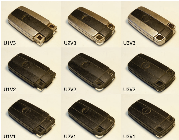
FIGURE 23. OVERVIEW OF ALL NINE 3-D PRINTED REMOTES SYSTEMATICALLY MANIPULATED IN UNITY ON THE X-AXIS (THROUGH EMERGENCE OF THE BUTTON AND CONTINUITY OF FORM) AND VARIETY ON THE Y-AXIS (THROUGH SIMILARITY IN MATERIALS).
